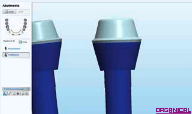
The shoulder of the bar structure is aligned to the abutment
