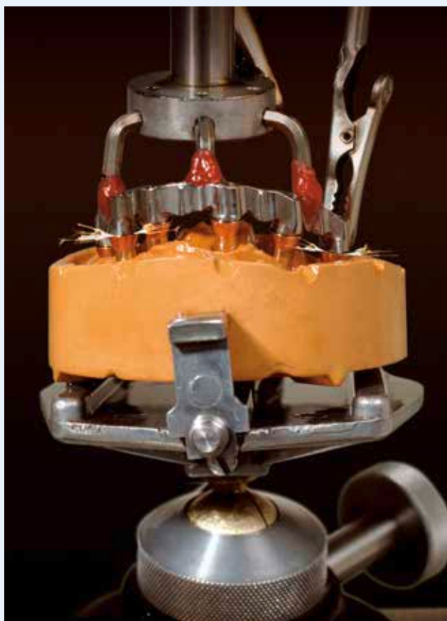
SAE spark erosion for the passivation of implant structures on abutments with standardised surface design.
