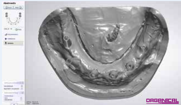
Scanned lower jaw model with SAE scan shells
